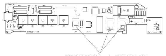
SWITCH POSITION on the KEYBOARD PCB
